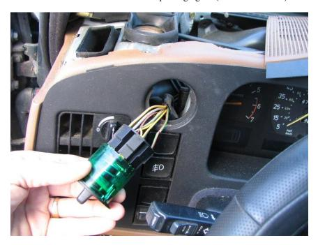
STEP 13 – Run Wires out to the aquarium for connection to the diagnostic connector I tried drilling a hole in the rubber plug but pushed it through by accident. I should have run it through where the large yellow wire is for my amp. I sealed with duct tape as best I could.
