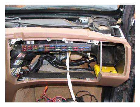
STEP 5 – Remove Anti Theft unit (slides out) This unit is from a 93. I believe the unit is different from 94 and newer.
