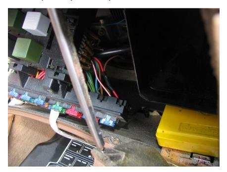
STEP 10 – Ignition switch connection (Red X on ignition switch) should be connected to the RED wire going to the right side of FUSE 27. I connected my  $2^{nd}$  Ignition wire from my remote to this. I added the Blue wire shown below.
