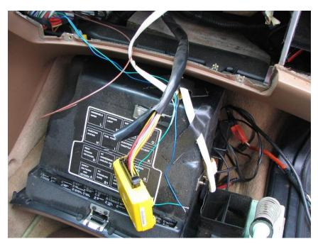
STEP 7 – Connect wires for Lock and Unlock These are the Yellow and Red wires located side by side toward the middle of the connector
